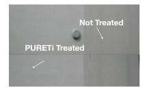
PURETi Clean is a spray applied, water based, light activated, pollution reversing, architectural surface treatment
